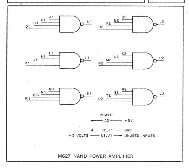
The M627 combines power amplification with high-speed gating, specifically for high fan-out of clock or shift pulses to expanded counters and shift registers. Propagation time between input and output transitions is typically 6 nsec. To utilize the timing accuracy of this module, wire runs of minimum length are recommended.
