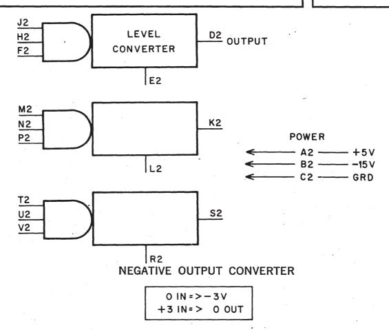
The M650 contains three non-inverting signal converters which can be used to interface the positive logic levels or pulses (of duration greater than 100 nsec) of K and M series to DIGITAL negative logic levels of —3 volts and ground. These converters provide current drive at a low output impedance so that unterminated cables or wires can be driven with a minimum of ringing and reflections.
