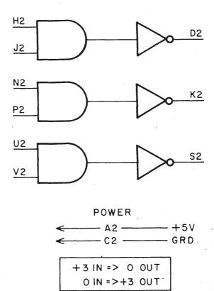
The M660 Cable Driver consists of three circuits each of which will drive 100 ohm terminated cable with M Series levels or pulses whose duration is greater than 100 nsec.
