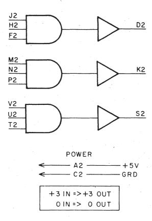
The M661 contains three circuits which may be used to drive low impedance unterminated cable with M Series logic levels or pulses whose duration is 100 nsec or greater.
