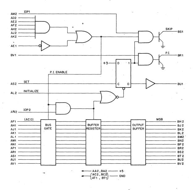
The M737 12-Bit Bus Receiver Interface is completely contained on a double height, single width module.
