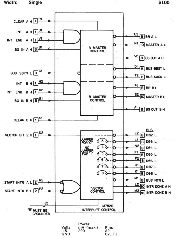
The M7820 is used in PDP-11 device interfaces. It consists of logic circuits that can be divided into three functional sections: Master Control A, Master Control B, and INTR Control.
