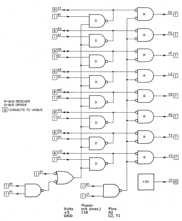
The M785 consists of eight drivers and eight receivers for use as a device interface with the PDP-11 UNIBUS. Pin U1 provides +3 volts and has an output capability of 10 TTL loads. Driver gates have open collectors and are capable of sinking 50 mA with a collector voltage of less than 0.8 volts.
