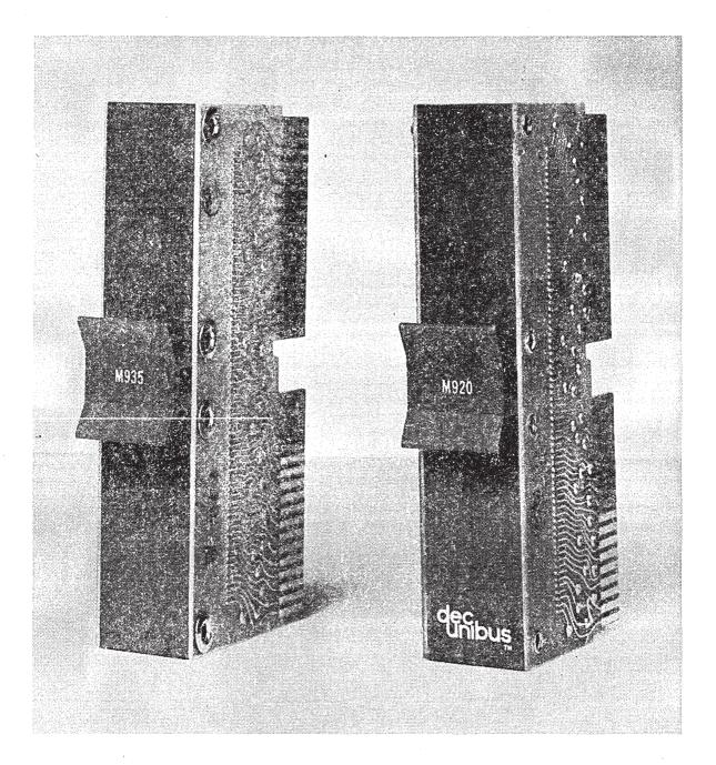
UNIBUS Jumper Module M920—The M920 Module is a double module that connects the UNIBUS from one system unit to the next. The printed circuit cards are on one-inch centers. A single M920 Module carries all 56 UNIBUS signals and 14 grounds.
