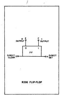
The R200 is a basic flip-flop for use in set-reset applications. It can be set and cleared at any frequency up to 2 mc. A set input makes the 1 output go to—3v and the 0 output to ground; a clear input makes the 0 output go to—3v and the 1 output to ground.
