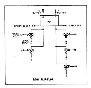
The R201 Flip-Flop has direct set and clear inputs and five diode-capacitor-diode (DCD) gates. Because of this large number of inputs, the R201 can be used in any of the following applications without additional gating:
