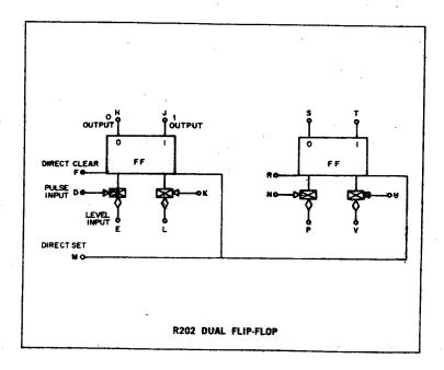
The R202 Dual Flip-Flop contains two identical flip-flops. Each has a direct clear input, a common set input, and two DCD gates. The R202 can perform in any one of the following applications without additional gating: up counter, down counter, shift register, ring counter, jam transfer buffer, and switch tail ring counter.
