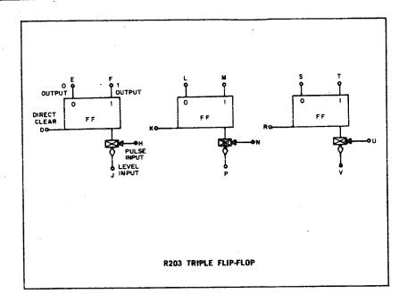
The R203 Triple Flip-Flop contains three identical flip-flops. Each flip-flop has a direct clear input and a DCD gate for conditional read-in.
