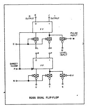
The R205 contains two identical flip-flops with a common direct clear input. Each has three DCD gates, and can be collector-triggered at either output by a diode-transistor gate or a diode network. The R205 can be used in any of the following applications without additional gating: up counter, down counter, shift register, ring counter, or jam transfer register.
