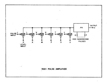
The R601 is a pulse amplifier that standardizes pulses in amplitude and width. Outputs may be either standard 100- or 400-nsec pulses (—3v to ground). It has six DCD gates so that inputs from as many as six sources may be mixed. Input pulses can occur at any frequency up to 2 mc for 100-nsec pulse outputs and up to 1 mc for 400-nsec outputs. Delay through the pulse amplifier is approximately 50 nsec.
