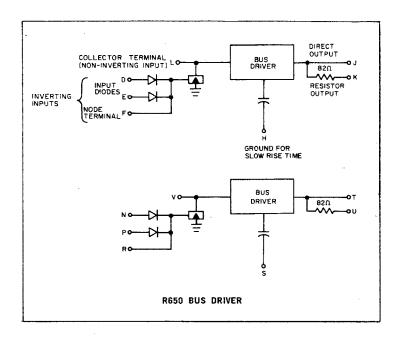
The R650 contains two inverting bus drivers for driving heavy current loads to either ground or negative voltages. The four input terminals make the R650 a versatile logic element as well. The diode inputs D and E (N and P) are the principal inputs. They form a NAND gate for negative inputs or a NOR gate for ground inputs. Gate inputs, such as the R001 or R002, can be added through the node terminal F (R). Other gating sources may be mixed with the gate inputs by using collector terminal L (V).
