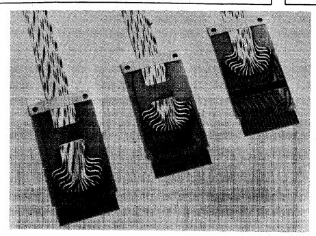
The W021, W022, and W028 provide cable connections to the FLIP CHIP mounting panel. The cable is a 19-conductor ribbon with nine signal leads and ten shields. The signal leads are connected to pins D, E, H, K, M, P, S, T and V. The shields are internally connected together and to pins C, F, J, L, N, R, and U.
