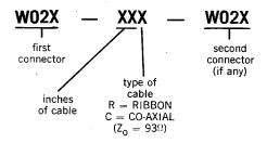
EXAMPLE: W028-24C two feet of co-axial cable attached, no second connector
