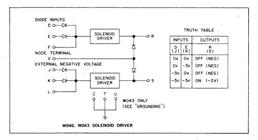
These high current driverscan drive relays, solenoids, stepping motor windings, or other similar loads. The output levels are -2 volts and a more negative voltage determined by an external power supply. One terminal of the load device should be connected to the external power source, the other to the driver output. There are two drivers per module and both modules use the same pin connections.
