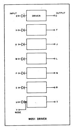
The W051 contains seven inverter amplifiers suitable for driving indicators, relays, and other medium power devices. The amplifiers can supply up to 100 ma at ground, and each output is diode clamped to -15v to prevent overvoltage when the current is interrupted in an inductive load. If the input is at -3v, the output is at ground.
