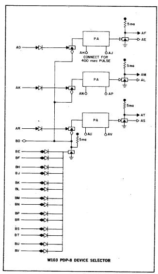
This module is used to decode the six device selector bits transmitted in complement pairs on the PDP-8 or PDP-8/S 1/0 bus, and it provides standard pulses to the selected device. The device code is selected by cutting one diode of each pair, BE or BF, etc., off the board. Device coding can also be accomplished by selective wiring of the bus inputs to the diode pairs.
