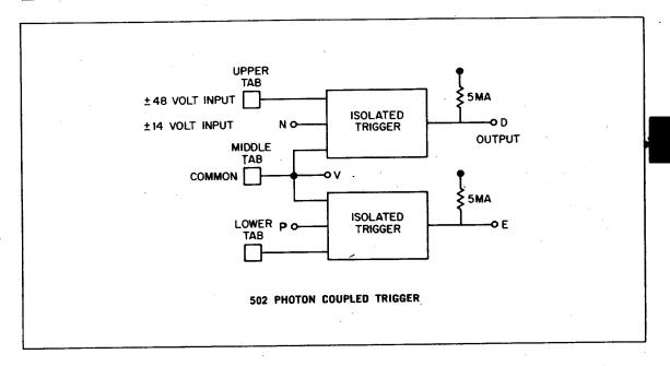
This special interface module allows process control system 48 volt signals to be transmitted to a digital control over long distances and despite floating supplies and noise. Additional low voltage inputs permit use as a pushbutton input device. Inherent delay in the photon-coupled isolation circuit filters out contact bounce. High voltage connections are at the handle end of the module to optimize isolation.
