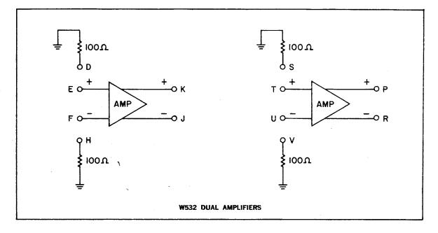
The W532 contains two AC-coupled differential amplifiers for use with many magnetic sense systems, including the H201 core memory. These amplifiers provide the high differential gain and common mode noise rejection necessary to amplify information signals in a system using a single sense line per plane for a memory or per channel for a tape system.
