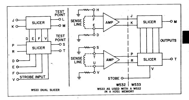
This module is used to detect amplified magnetic system sense signals from a W532 (see above diagram) and convert them to positive DEC pulses. Detection of signals as narrow as 100 nsec is possible over a wide range of detection thresholds. There are two slicer circuits on each W533. Two input terminals per circuit permit rectification so that bipolar difference signals can be sliced and standardized.
