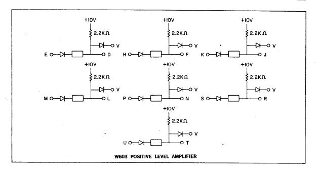
Positive logic systems such as those using RTL, DTL, or TTL monolithic integrated circuits can be driven from FLIP CHIP systems through the W603. Clamped load resistors at the output of each circuit permit output levels to be adjusted to the type of circuit being driven. Normally the clamp voltage at pin V is provided by the logic supply voltage used with the monolithic circuits. This clamp voltage is common to all seven converters on the module.
