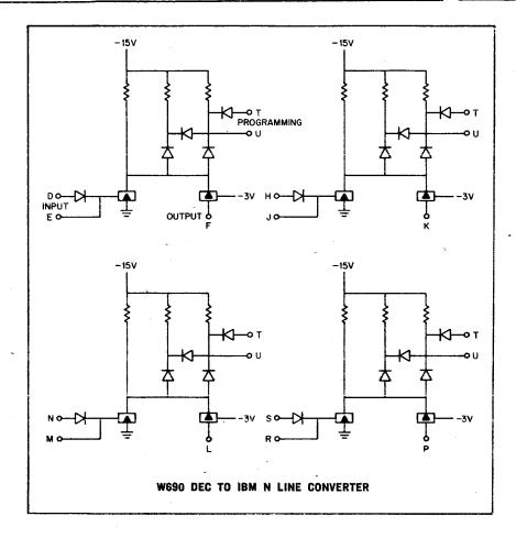
Each of the four inverting drivers on this module provides outputs compatible with the three types of IBM N lines, depending upon what output currents are programmed by grounds or open circuits at pins T and U. Node points are provided at each input. Maximum delay: 100 nanoseconds driving N transmission lines.
