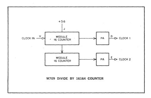
The W709 module provides the count-down circuitry for conversion of stable crystal clock frequencies to low frequencies common to teletype and data communications systems.
