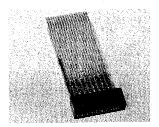
The W980 Module Extender allows access to the module circuits without breaking connections between the module and mounting panel wiring.
