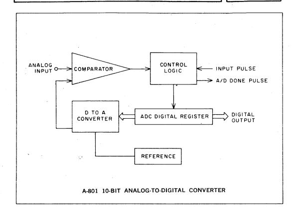
The A-801 is a complete, 10-bit, successive approximation, analog to digital converter with a built in reference supply. The complete converter is contained on one DEC double FLIP CHIP™ logic module. Conversion is initiated by raising the Convert input to logic 1 (+4 volts). The digital result is available at the output within 10 microseconds. An A/D Done Pulse is generated when the result is valid. The A-801 uses monolithic integrated circuits for control logic, output register, and comparator.
