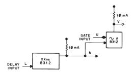
The B312 is an adjustable delay line with suitable buffering driving a standard 2 mA diode gate. The delay is set by a screwdriver adjustment accessible from the handle end. This module has the same pin connections and can be used in the same slot as the B311 tapped delay line module.
