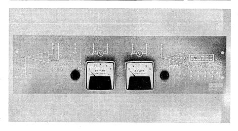
This panel provides facilities for experimenting with analog-digital techniques. It contains a 4 bit variable output D-A converter and a comparator circuit. Also includes two 8 volt panel meters and a potentiometer for producing 0 to —8v test signal. Connections to these devices are made with Type 911 Stacking Banana-Jack Patchcords.
