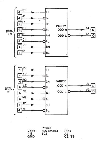
The M162 contains two parity detector circuits. Each circuit indicates whether the binary data presented to it contains an ODD or EVEN number of ONES. The data and its complement are required as shown.
