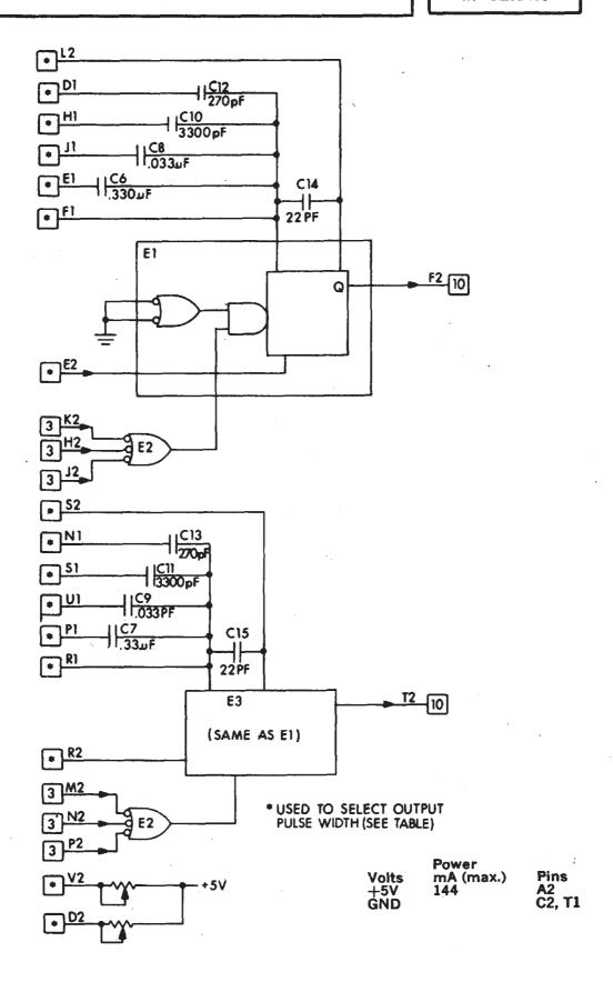
The M3020 Module contains two monostable multivibrators, each of which is activated by the output of a Schmitt Trigger circuit. A low input transition on any one of the three inputs to the Schmitt Trigger circuit produces a positive output pulse and triggers the multivibrator. The Schmitt Trigger circuit provides a hysteresis current which prevents the multivibrator from being triggered erroneously by noise signals at the input.
