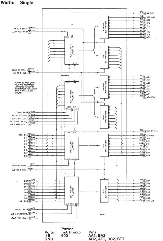
The M795 Word Count and Bus Address Module is used to interface Direct Memory Access (DMA) devices to the UNIBUS. This module contains two 16-bit counters. One counter is used to count the number of data transfers that occur. The other counter is used to specify the bus address of the data to be transferred.
