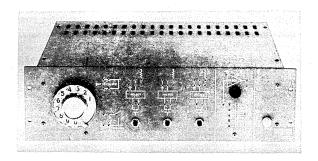
The Type 900 Control Panel uses the same chassis and input controls as the 700D but does not contain a power supply. It is designed for multistudent installations of DEC Logic Laboratory units powered by a single 700D Power Supply. Connections are available on the rear of the 900 to accept power from the master 700D Power Supply.
