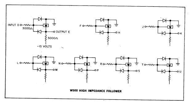
High impedance signal sources such as photocells and low-current instrumentation amplifiers can drive Schmitt Trigger W501 or logic gates through a W500 circuit. The module contains 7 fault-protected circuits, each comprising two cascaded emitter-follower amplifiers. Input voltage excursions up to  $\pm 30 \nu$  or short-circuits from output to ground are harmless. Outputs can go as negative as  $-15 \nu$  with very light loading, but will not exceed  $-10 \nu$  when driving a W501 input.
