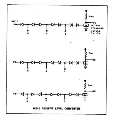
The Type W510 Positive Level Converter contains three circuits that convert positive levels to DEC standard levels of ground and —3v. Each circuit consists of a grounded-emitter inverter with a diode string between its input and the base of the inverter. By shorting out sections of the diode string, the switching threshold may be varied to either +2v,
