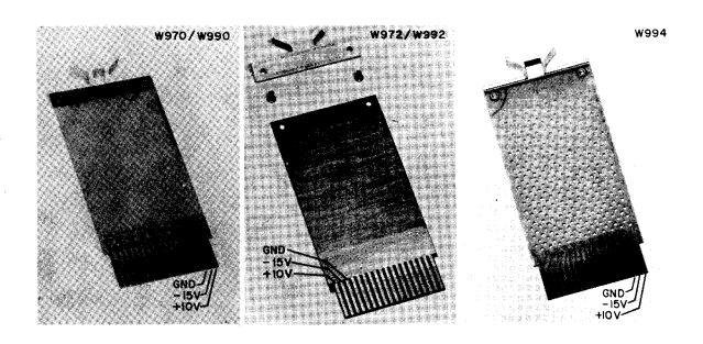
These 10 blank modules offer convenient means of integrating special circuits and even small mechanical components into a FLIP CHIP system, without loss of modularity. Both single- and double-size boards are supplied with contact area etched and gold plated. The W990 Series modules provide connector pins on only one module side for use with H800 connector blocks. W970 series modules have etched contacts on both sides of the module for use with double density connectors Type H803.
