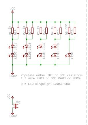
R1-R5 must be less than 2.4 mm thick.
