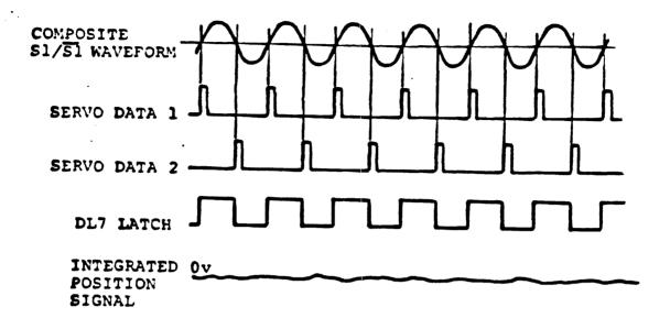
Figure 3 Integration of \$1/\$\overline{\$1}\$ Composite
