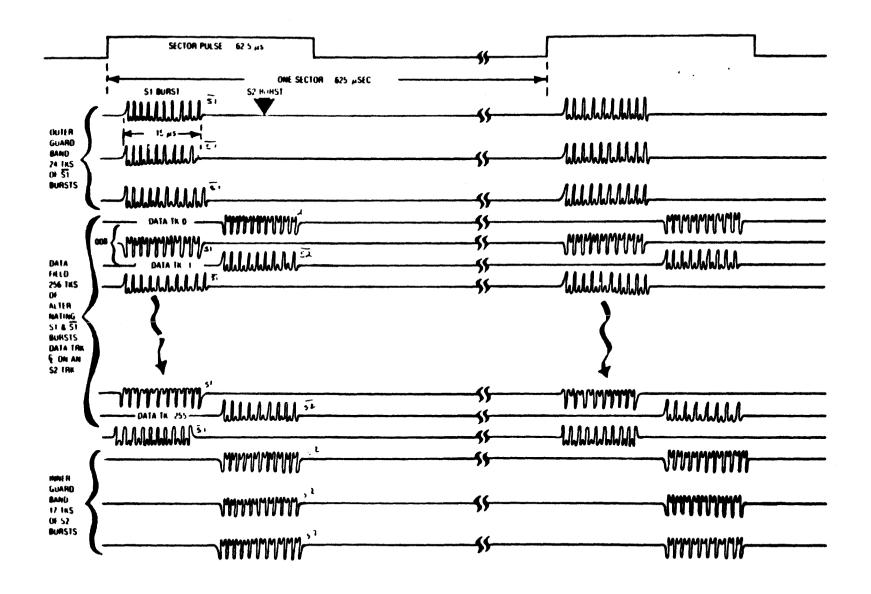
Figure 1 RL01 Servo Data Format
