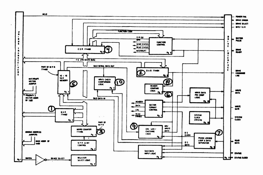
Figure 7 M7762 RL11 Basic Block Diagram
