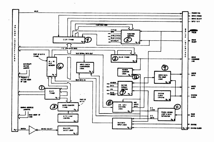
Figure 6 M7762 RL11 Basic Block Diagram
