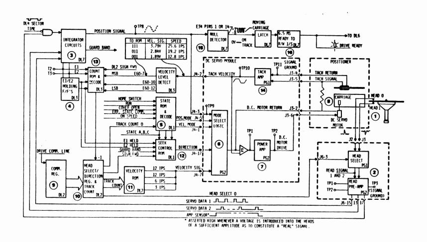
Figure 2 Track — Following Servo Block Diagram
