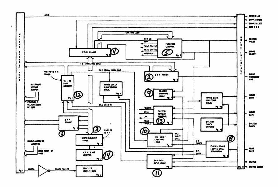
Figure 5 M7762 RL11 Basic Block Diagram
