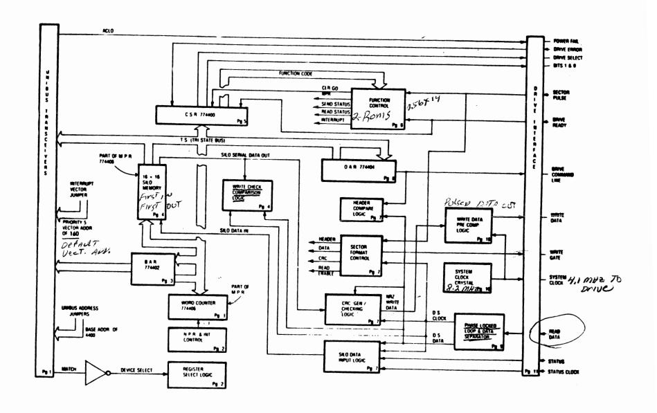
Figure 2 M7762 RL11 Basic Block Diagram
