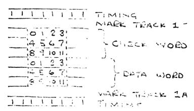
Notice that the data word is recorded as indeed, as a "check word". The numbers that styre is the site of the data word. The data word and sheck word are neglically ORed together to prevent "bit dropout".
