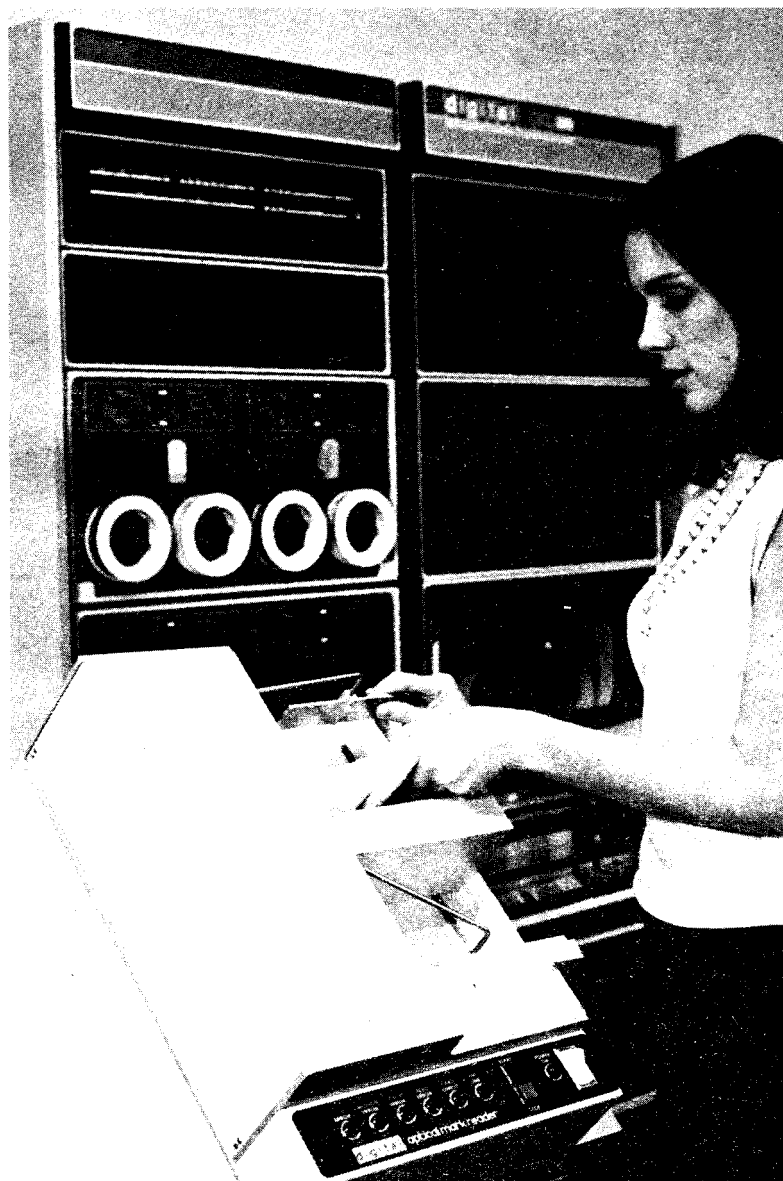
DEC offers the CR8-E Card Reader and Control Option and the CM8-E Optical Mark Card Reader and Control Option.
