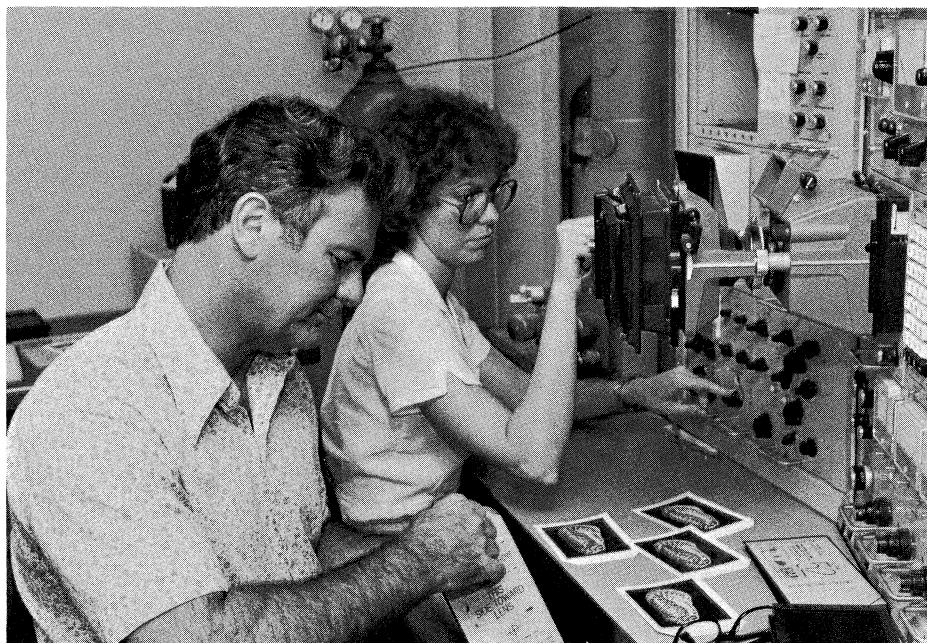
Fig. 2. Dr. Benson and an assistant photograph ostracode specimens on a Scanning Electron Microscope. This is one of the first steps in the procedure to analyze these microscopic creatures using the 4052.
