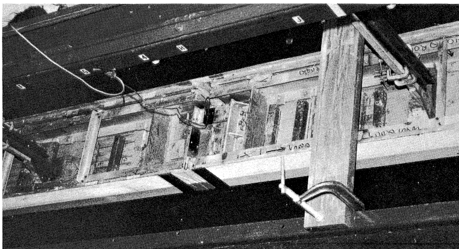
Figure 2b. Sensors on the midsection of the model pick up its bending moment. Dr. Armin Troesch is making some adjustments to the instrumentation.
