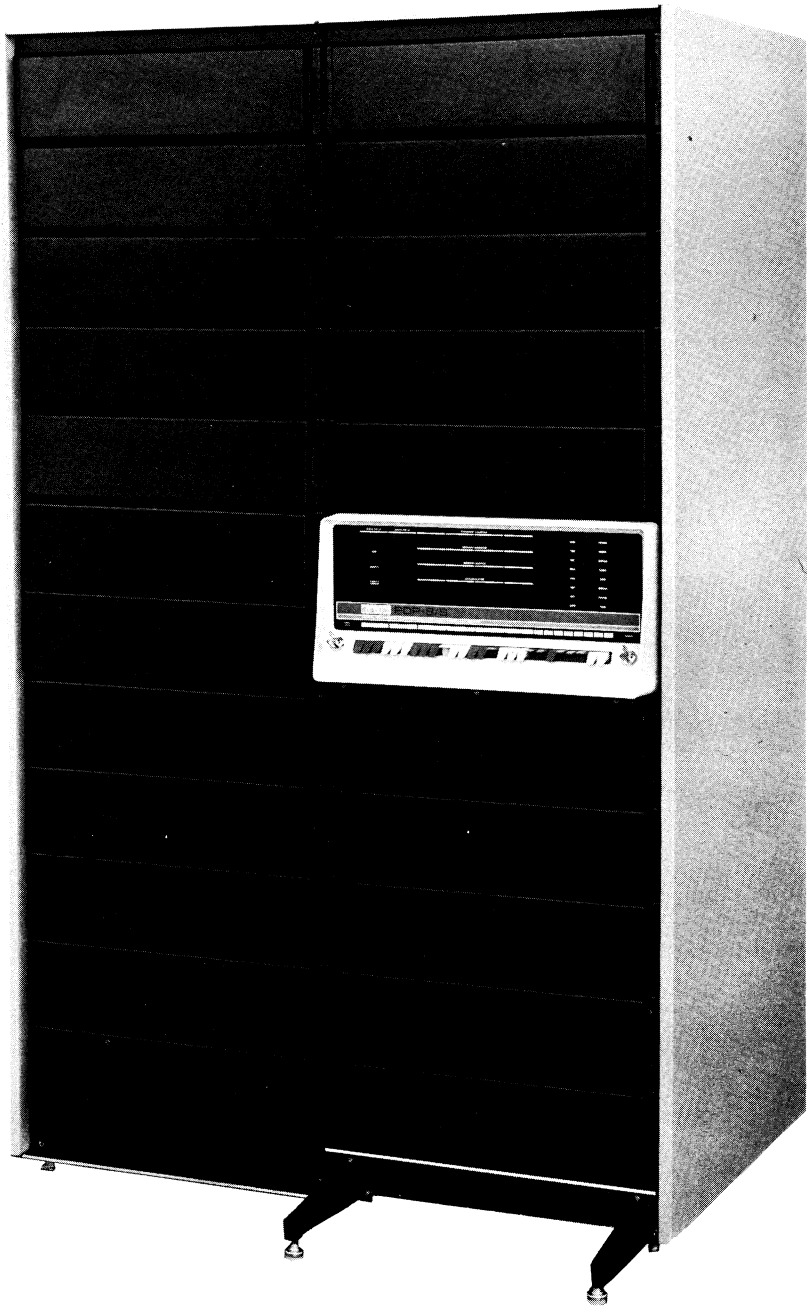
Typical PDP-8/S and Disk File Installation
