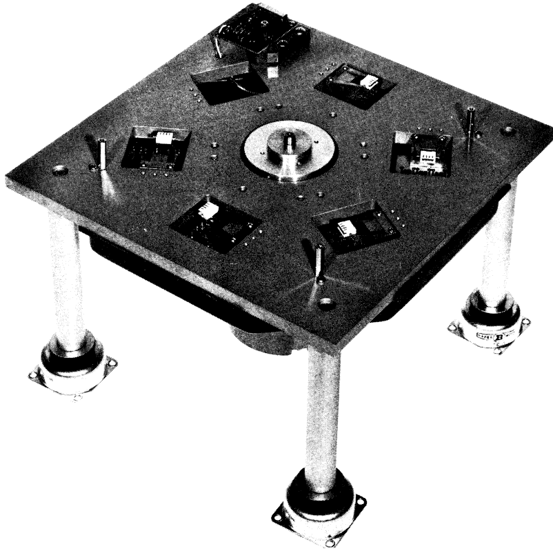
Figure 1-4 Disk File Assembly, Read/Write Head Locations
