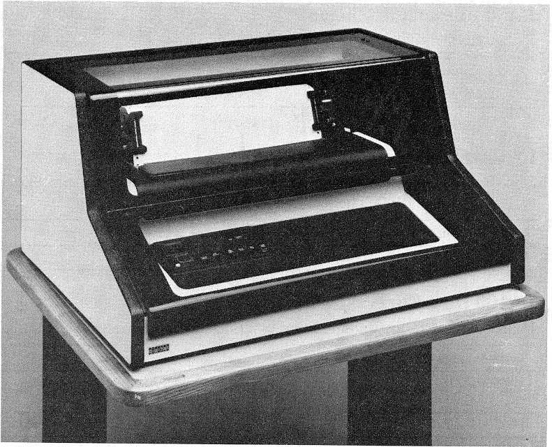
Figure 8-6 LA100 Acoustic Cover
