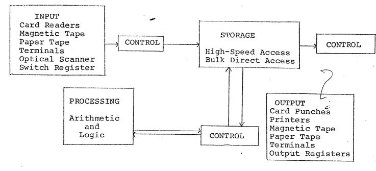
One of the earliest forms of computer I/O was paper tape. These systems were very slow for program development, and the file structures (boxes and racks of paper tape) were bulky and unreliable. On the PDP8, versions of BASIC, FOCAL, and Assembler used this method.
