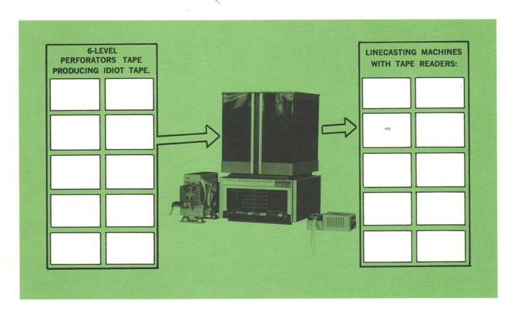
The PDP-8 Typesetting System accepts idiot tape as fast as 10 to 12 keyboard operators can produce it on Flexowriters or any other 6-level tape perforators. It turns the idiot tape into hyphenated/justified tape at a rate of 12,000 lines per hour — enough to keep 10 to 12 linecasting machines busy.
