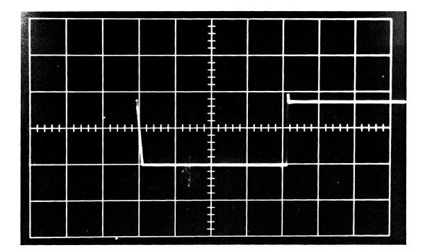
Figure 5-6 Read (or Write) Delay
