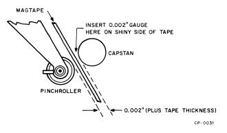
Figure 5-3 Pinchroller – Capstan Clearance
