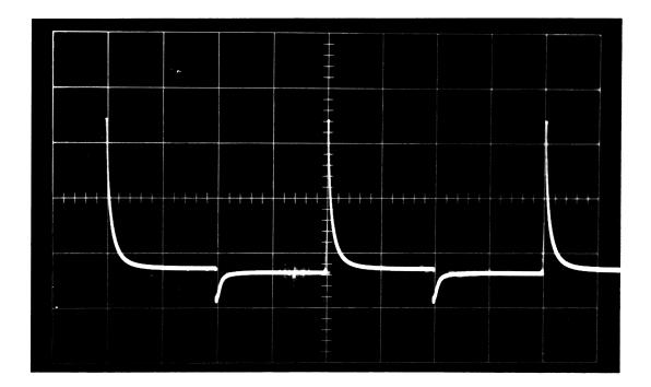
Figure 5-5 Write Driver Output
