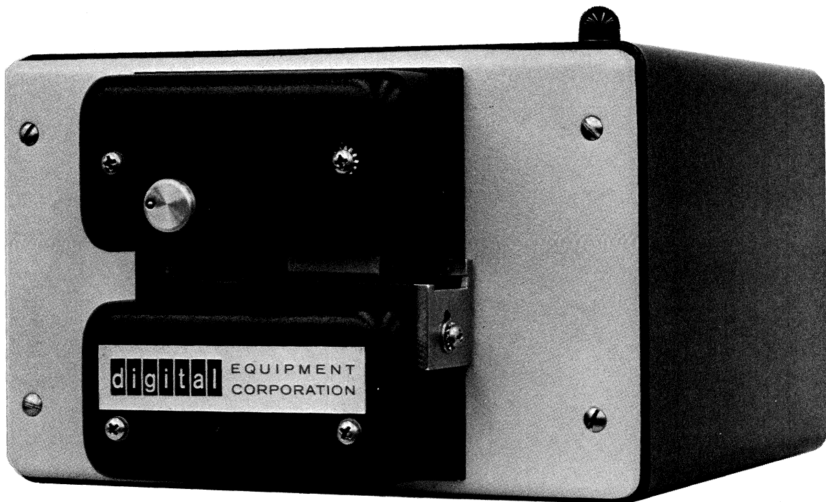
Figure 1-1 PR68A High-Speed Paper-Tape Reader
