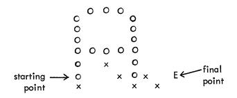
The "o" indicates an intensified point, the "x" a nonintensified point, and "E" the point at which the escape is given.
