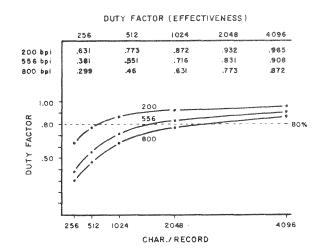
Note that these rates could never be realized in practice with a double-buffer type of throughput since the assumption of the necessity of a double buffer implies that at least two records-an ideal case and therefore one interrecord gap-will be written.
